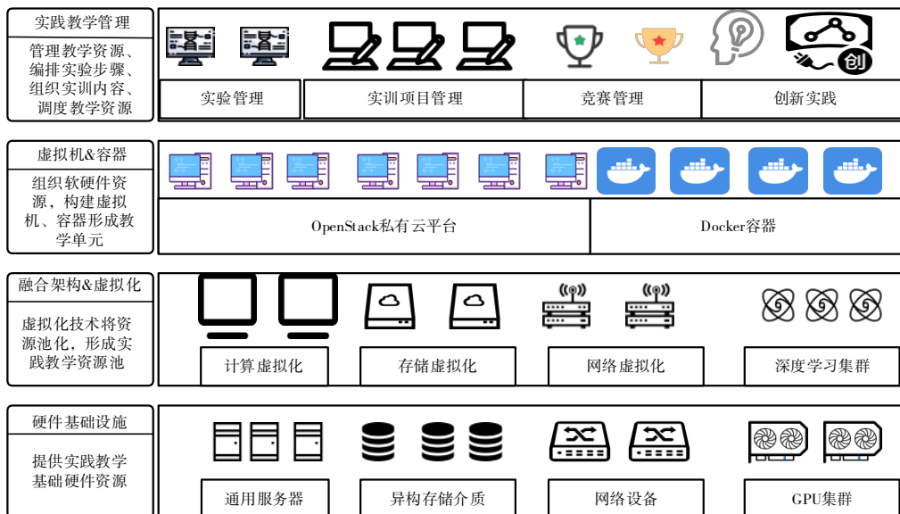
Fig. 2 Architecture of the innovative practical platform 图2 创新实践平台架构
